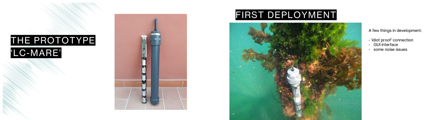
Figure 4. (Left) Photograph of prototype low-cost underwater acoustic recorder and its waterproof housing. (Right) Photograph of prototype low-cost underwater acoustic recorder in situ. Figure from Lucille Chapuis, La Trobe University.
