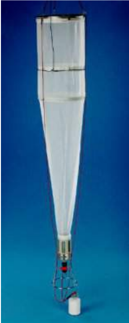
Figure 4: Indian Ocean Standard Net developed for the International Indian Ocean Expedition.
