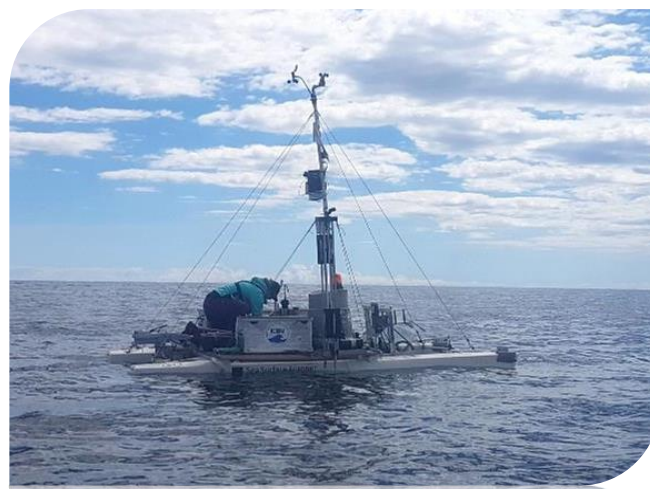
Figure 9: Our Catamaran "Sea Surface Scanner" which can collect in situ data on the SML and ULW at 1 m and can collect discreet water samples. Featured being deployed in the Baltic Sea. © Oliver Wurl
