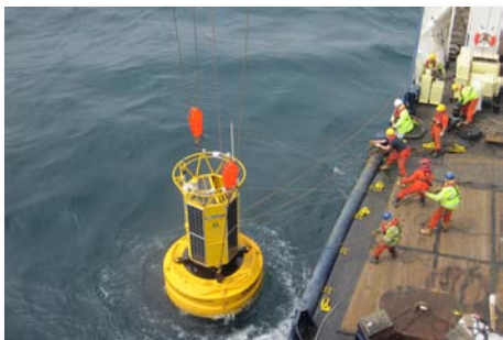
New buoy for the Western Channel Observatory Photo Credit: PML
