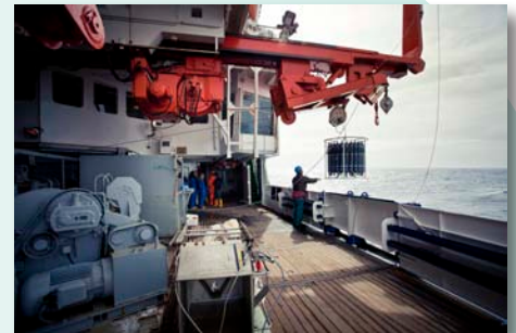
A member of the Polarstern crew lowers the CTD probe into the depths. Photo: Thomas Steuer, Alfred-Wegener-Institut
