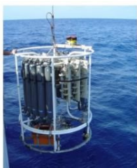
Microstructure turbulence measurements with an MSS90L (Sea & Sun Technology) during the MOSAiC campaign. Image credit: Lisa Grosfeld, Alfred Wegener Institute
