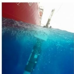
Microstructure turbulence measurements with an MSS90L (Sea & Sun Technology) during the MOSAiC campaign. Image credit: Lisa Grosfeld, Alfred Wegener Institute
