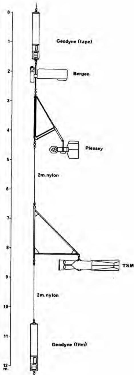
Figure 3 Enlarged diagram of relative positions and sizes of current meters in SCOR-21 moorings
