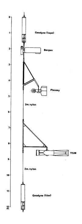
Enlarged diagram of relative positions and sizes of current meters Figure 3  $$\rm in\ SCOR\text{-}21\ moorings$$
