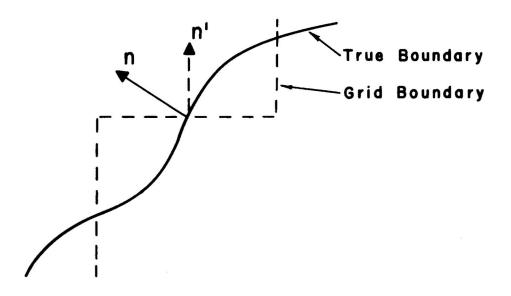
approximating the true boundary, the boundary condition should be  $v_n=0$ , not  $v_{n'}=0$ . (iv) there is some question as to whether the LaPlace equation applied to a bumpy bottom gives the appropriate scattering condition for surface tides in the pressure of internal stratification.
