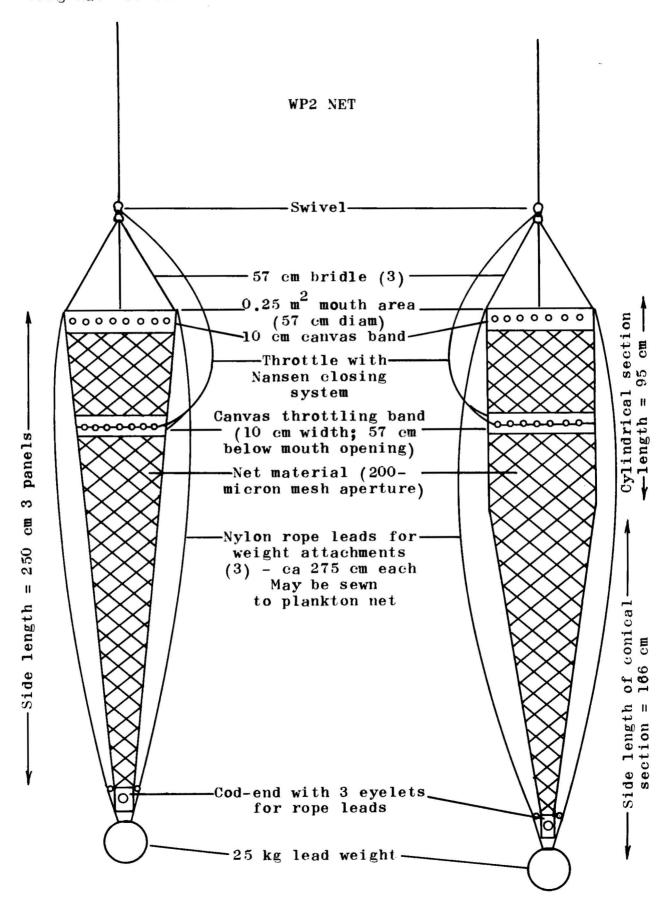
b) Where plankton is rich, and is not required living, a detachable cod-end bag of the same mesh as the net is more convenient to handle than a bucket.
