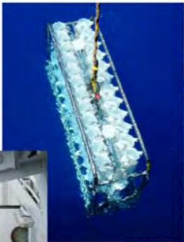
Coated stainless steel torpedo (FISH) for trace metal clean surface sampling
