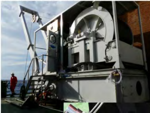
The NIOZ Kley France winch with A frame and 10 km trace metal clean kevlar cable for CTD deployment on the RRS James Cook
