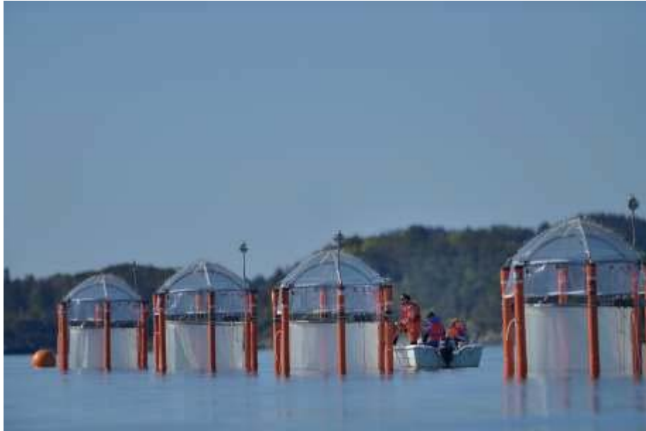
Figure 4 Large volume mesocosms of 20 m depth deployed in the Raunefjord, Norway to investigate the impacts of ocean acidification on pelagic communities (photo: Solvin Zankl, GEOMAR, 2015)
